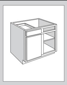
Blind Corner Base cabinets are 341/2" high by 24" deep. The visible width of these cabinets ranges from 13 %" to 28" wide.
