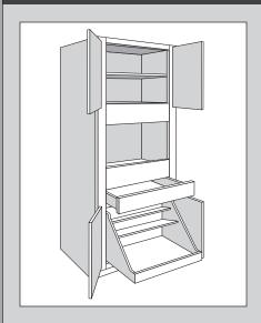
Oven cabinets range in size from 27" to 33" wide, from 84" to 96" high and are 24" deep.
